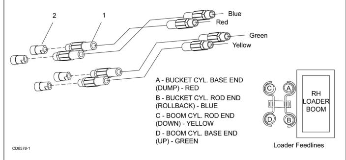
Figure 6. Loader Feedline Connections
